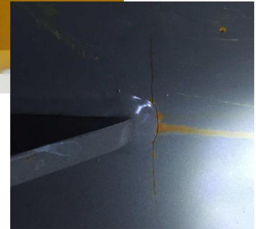
fatigue crack at end of rib
